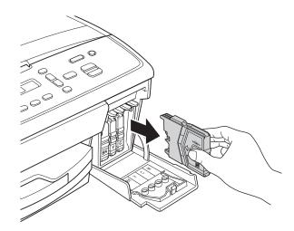
Open the new ink cartridge bag for the colour indicated on the LCD, and then take out the ink cartridge.
